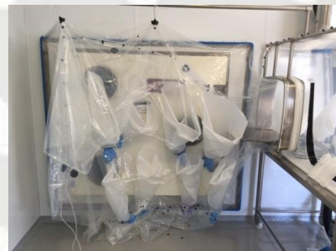
Flexible enclosure attached around Dryer
