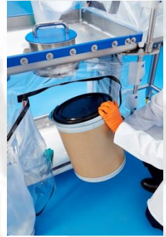
Drum entry via lift platform
