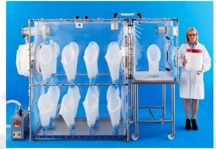
Floor Tray isolator for wheel in granulation equipment
