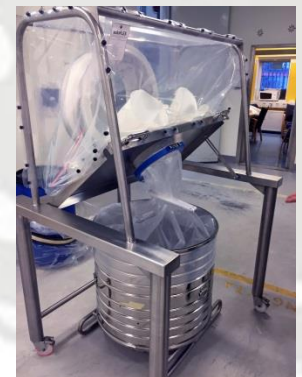
DT with hinge up base for easy bin liner attachment
