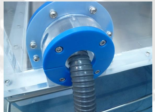
Gas tight utility port
